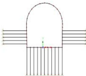
Figure 3: The tunnel lining simulation with linear elements using SAP 2000 [5].
