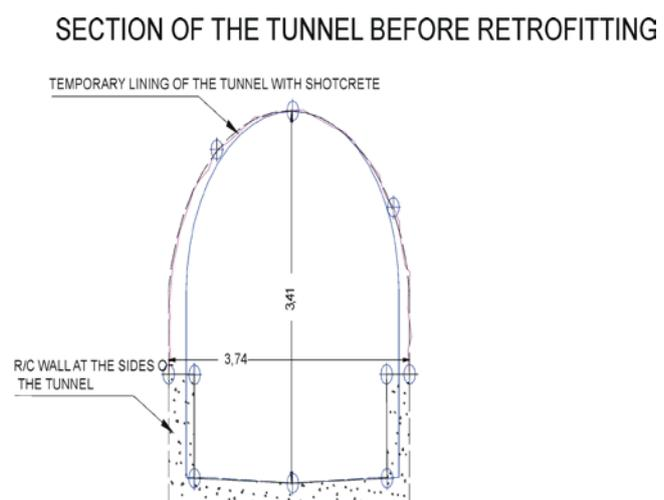
Figure 2: Typical section of the tunnel with shotcrete lining that suffered failures.
