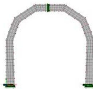
Figure 5: Simulation of *polygonal* tunnel lining using Lusas 14.7 [6].
