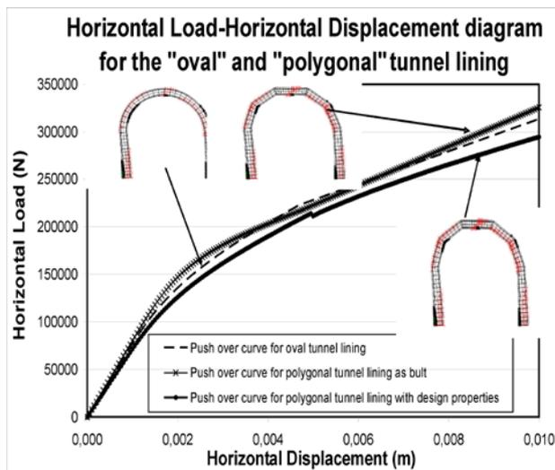
Figure 7: Horizontal load-displacement diagram for the oval and polygonal tunnel lining with failure pattern.
