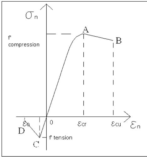
Figure 6: Stress-strain curve for the simulation of plane stress elements representing concrete.
