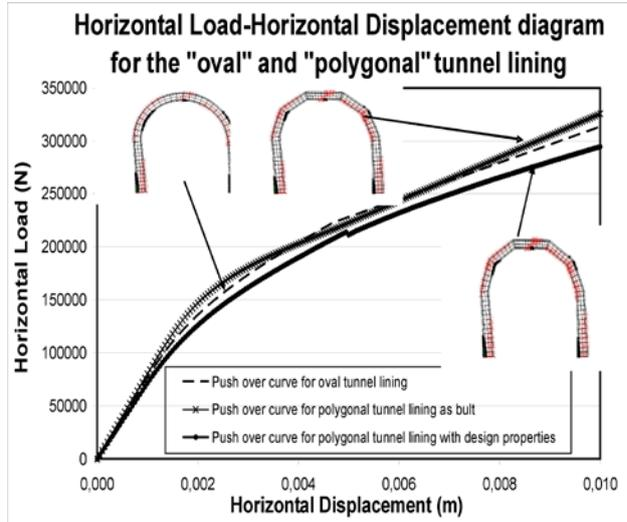
Figure 7: Horizontal load-displacement diagram for the oval and polygonal tunnel lining with failure pattern.
